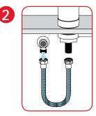
Connect to cold water inlet using the HOTAP water inlet hose
