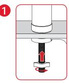
Place HOTAP over the tap hole and tighten mounting nut to secure the faucet
